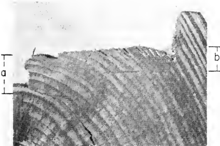
Section at Field End of Tie Plate
